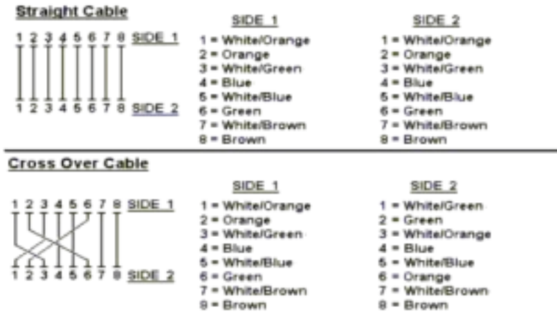
Figure A-1: Straight-Through and Crossover Cable
